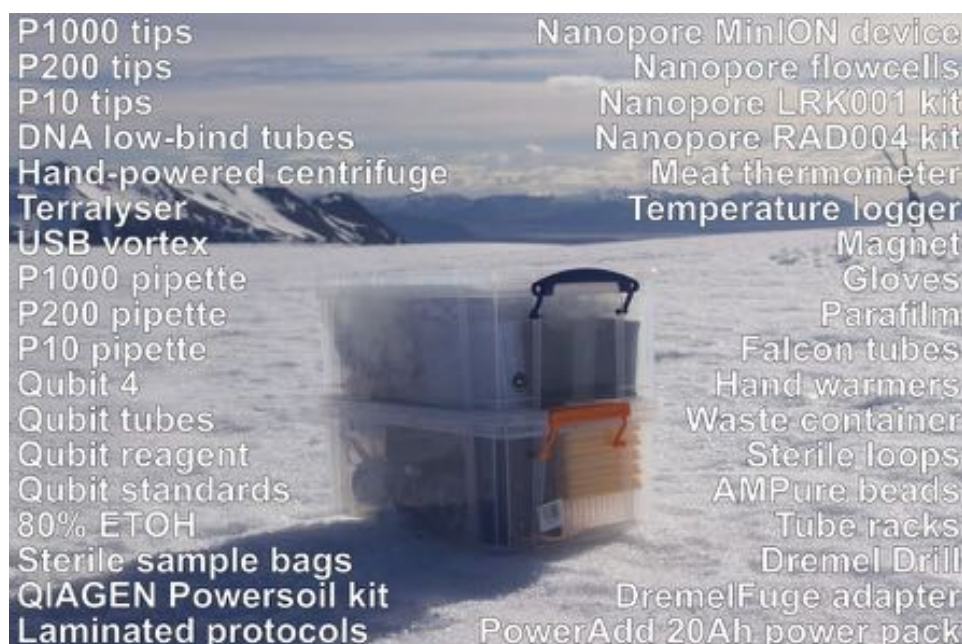
The contents of our 2x 9L boxes comprising the majority of the SledgeLab
