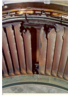
Figure 1.4: Example of turbine blade failure from blade vibration
