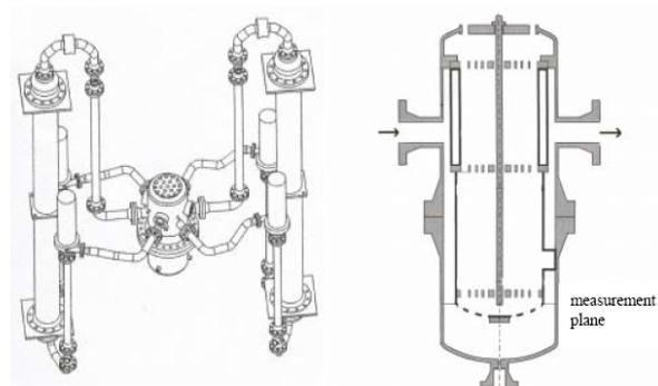
Scaled down model of a Babcock & Wilcox (B&W) PWR with height ratio of 1:4.
