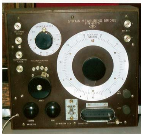
Fig. 21 A Tinsley Wheatstone strain gauge bridge, here with built in galvanometer, bottom right Now in the Kirkaldy Testing Museum
