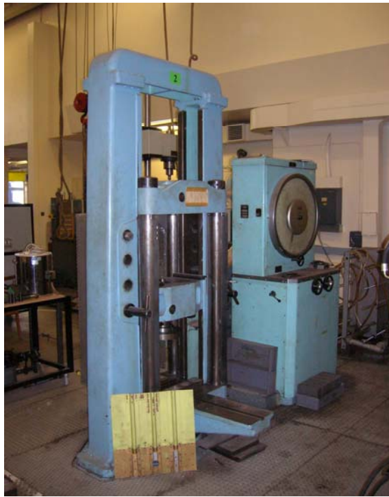
Fig.13 The 100t (c 1MN) Avery testing machine for the Transit Camp in 1955, here pictured in the Heavy Testing Lab on level 1 of E3, in 2007 (photo courtesy Hugh MacGillivray)
