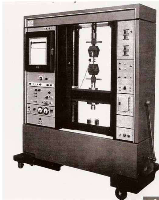
Fig. 15 A 10.000kN (c 10t) Instron as installed in the Poylymer lab and later in lab 581.
