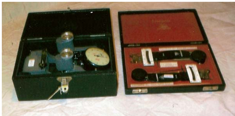
Fig. 22 A 2in Lindley dial gauge extensometer and a pair of 1in Huggenberger tensometers. demonstration and to allow long term readings to be taken by the Civil department of certain settlement strains in the structure. I do not know when such readings ceased. There were several resistance strain gauge measuring circuits - two Savage & Parsons 50 channel static strain gauge bridges (one from Waterhouse and Transit Camp days), two Tinsley static strain gauge bridges (one now in the Kirkaldy Testing Museum) and six channel switch box, dynamic strain gauge circuitry, some Philips 'carrier wave' circuits with high speed Kelvin Hughes pen recorders and some with drift corrected D.C. amplifiers and C.R.O display from Southern Instruments (all valve operated, in the days before chips and printed circuits); one or two inductive displacement 'pick-ups' and surely some instruments I do not now recall. A number of these strain gauge instruments were on more or less permanent loan to the already existing 3rd year/post-graduate lab in E2, including the Philips carrier wave bridge and a larger Kelvin & Hughes pen recorder for use on the electric hoist rig, as of Transit
