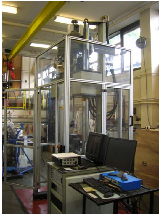
Fig.32 The Instron high speed impact machine with compressed nitrogen used to pressurise the hydraulic system. (Photo by courtesy of Hugh MacGillivray)
