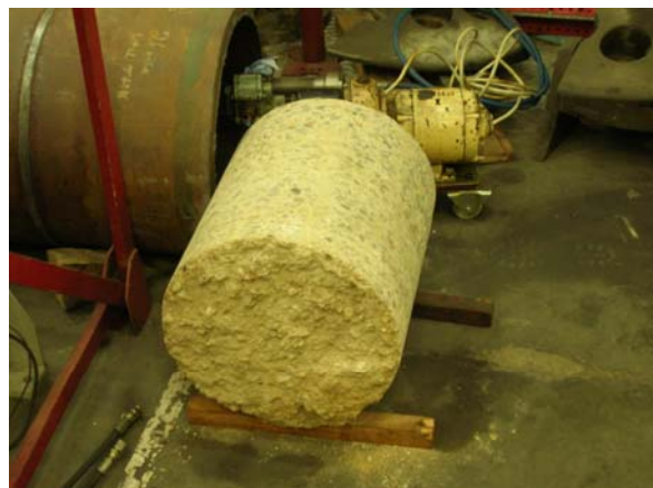
Fig. 34 Part of a reinforced concrete column cut from the E3 foundations, to be tested for its strength
