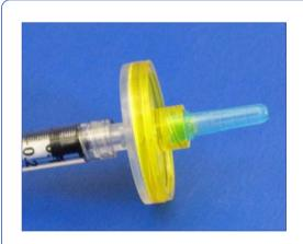
Over-pressurising syringe filters causes filter and syringe to separate.
