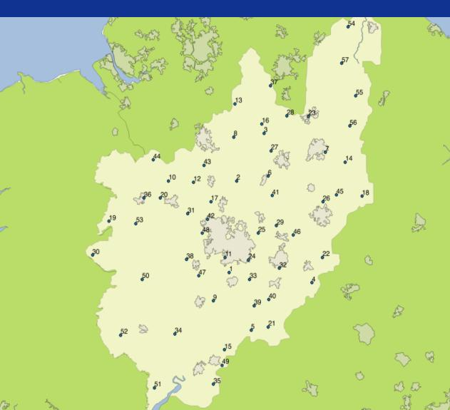
Regional Frequency Analysis, using an L-moment approach, is implemented on series of annual maxima on 57 selected sites within the Midlands area. A comparison with the traditional at-site estimation method is carried out, and an assessment of the accuracy and reliability of the estimates is performed using Monte Carlo simulation. Spatial interpolation of extremes at ungauged locations is also implemented in the form of contoured figures.
