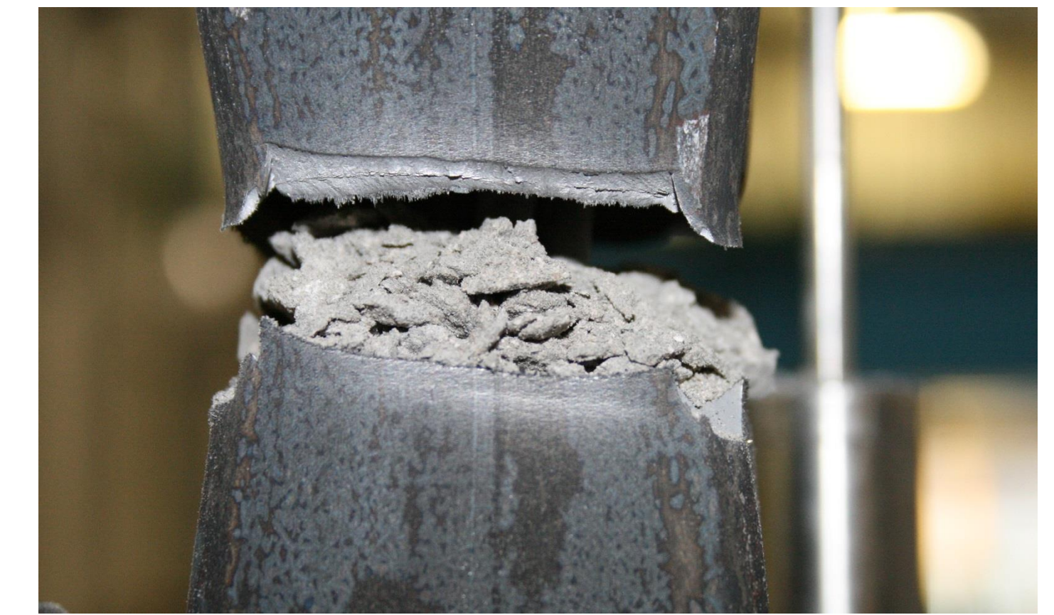
Figure 7: Failure of an S690 grouted specimen
