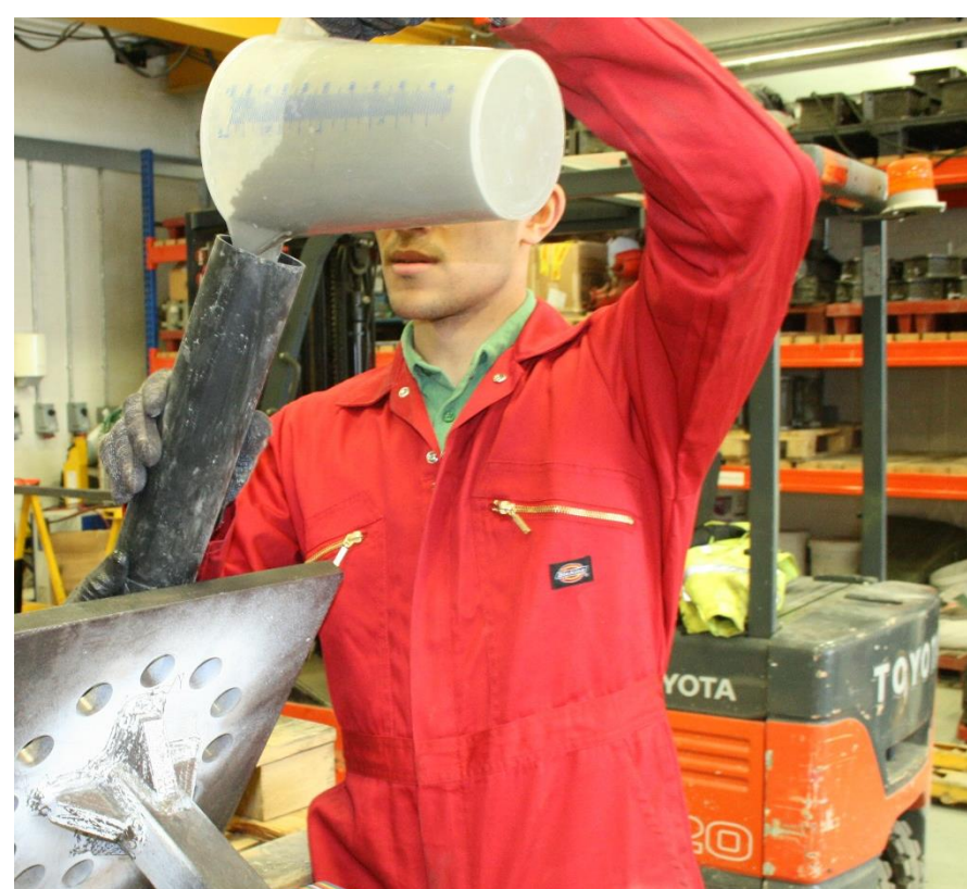
Figure 4: Pouring grout into specimen
