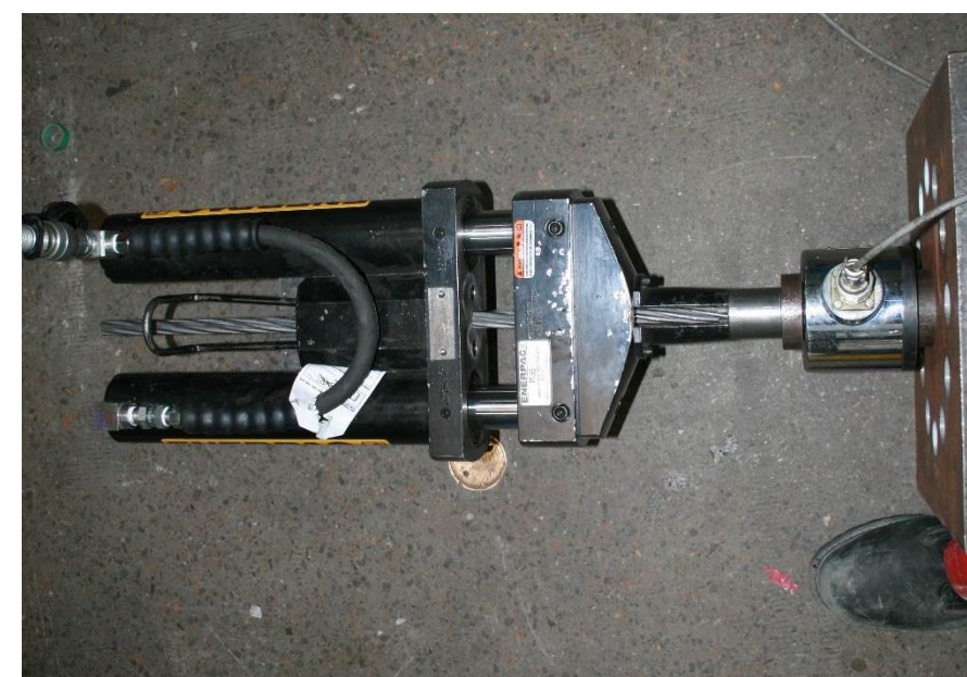
Figure 2: Stressing jack and cable
