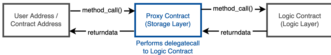
Figure 2.2: Standard Upgradeability Proxy Pattern
