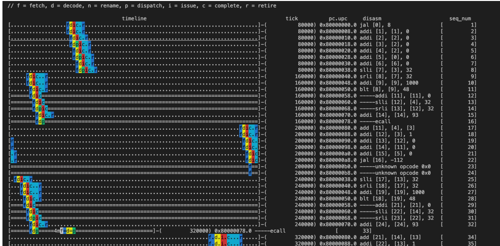
(a) Beginning of the pipeline after removing register renaming
