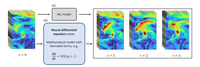
Figure 1: Workflow overview. Instead of using a purely data-driven ML model to simulate the weather and climate as shown by (a), in this project we will investigate using neural differential equations (NDEs) (b). The NDE defines a hybrid model which combines an existing mathematical model with learnable components.
