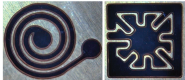
Figure 4 Masks produced in brass sheet. Masks are approximately 10 mm in width
