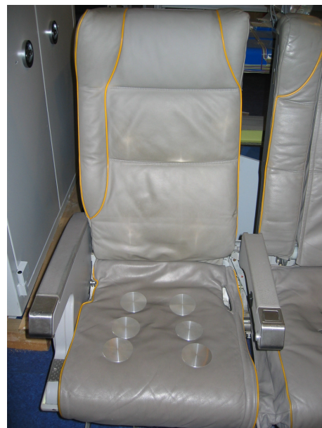
Figure 5: Infrared image (left) and installed demonstrator (right) of a static thermoelectric harvester for aircraft seat sensors [16].
