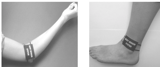
Fig 1 Examples of body movement detection; wireless sensor packs are provided at limb joints to monitor several motion parameters continuously.
