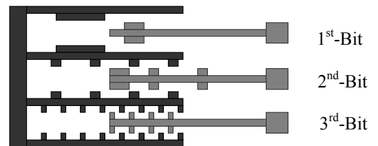
Fig 5 Schematic of a 3-bit digital comb drive.
