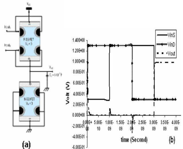
Figure 6: (a) Schematic circuit of a SGrFET NOR (b) NOR Output/Inputs Voltages vs. time
