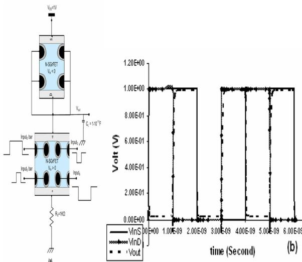
Figure 8: (a) Schematic circuit of a SGrFET XOR with triple unit cell driver (b) XOR Output/Inputs Voltages vs. time
