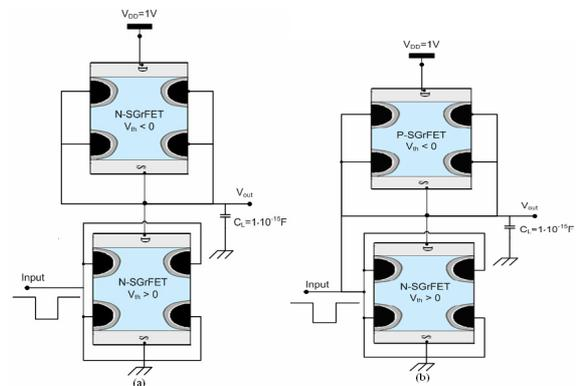
Figure 3: (a) n-SGrFET inverter, (b) C-SGrFET inverter.
