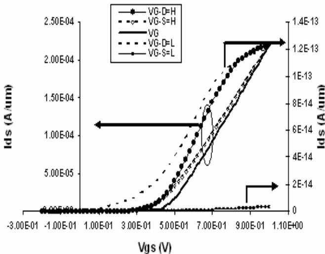
Figure2: Transfer characteristics of the DC sweep of one gate row with the other gate row voltage constant.  $V_{DS}=1\text{V}$ .
