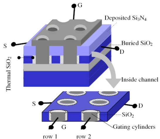
Figure 1: Schematic configuration of a SGrFET with two gating rows, each consisting of 3 gate cylinders.
