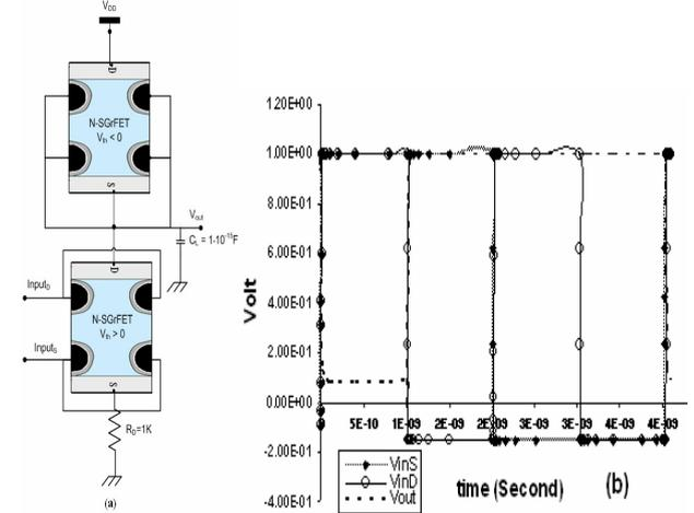
Figure 5: (a) Schematic circuit of a SGrFET NAND (b) NAND Output/Inputs Voltages vs. time
