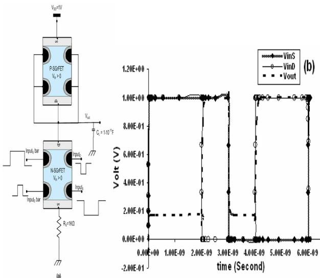
Figure 7: (a) Schematic circuit of a SGrFET XOR (b) XOR Output/Inputs Voltages vs. time
