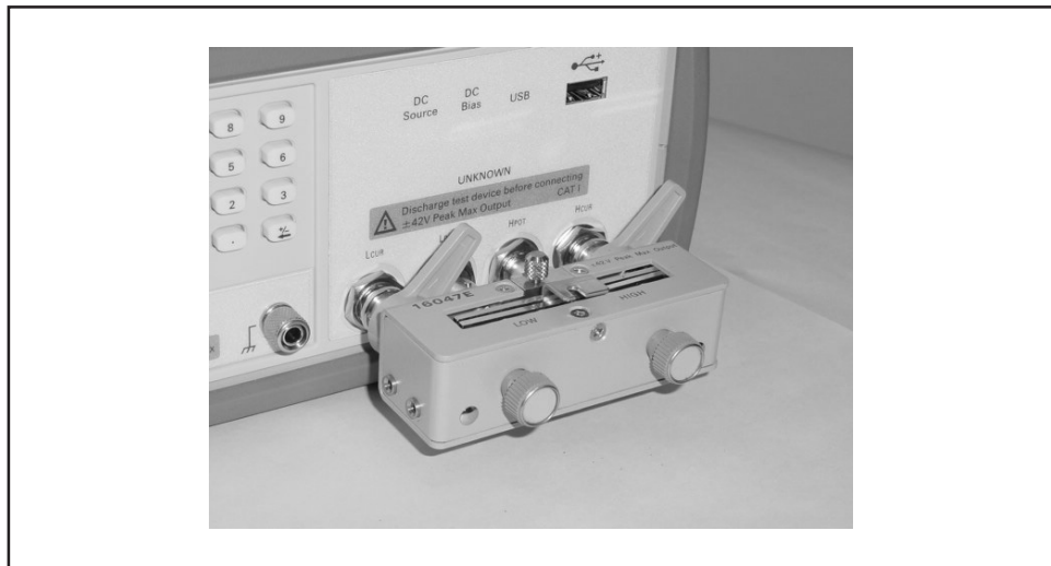
Figure 7-19 Connecting a shorting bar
