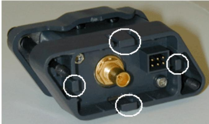
When installing an adapter on the instrument's connector panel, align the male 6-pin connector with the female connector and push the adapter straight in. There will be some resistance and you'll hear clicks as the four clips slide into place. Then tighten the captive screws.
