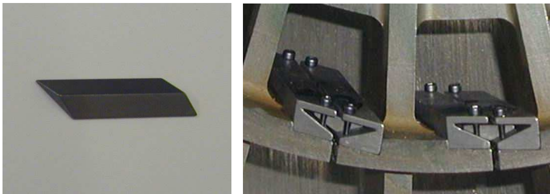
Figure 6.14 (a) a C-R damper, and (b) its installation in Blisk-1
