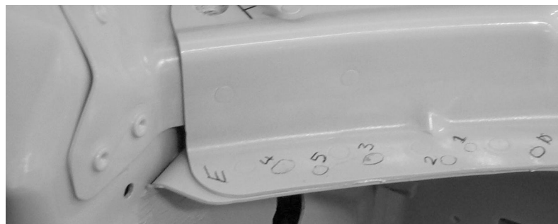
Figure 6-3 Example of bonded joint tested on automotive structure.
