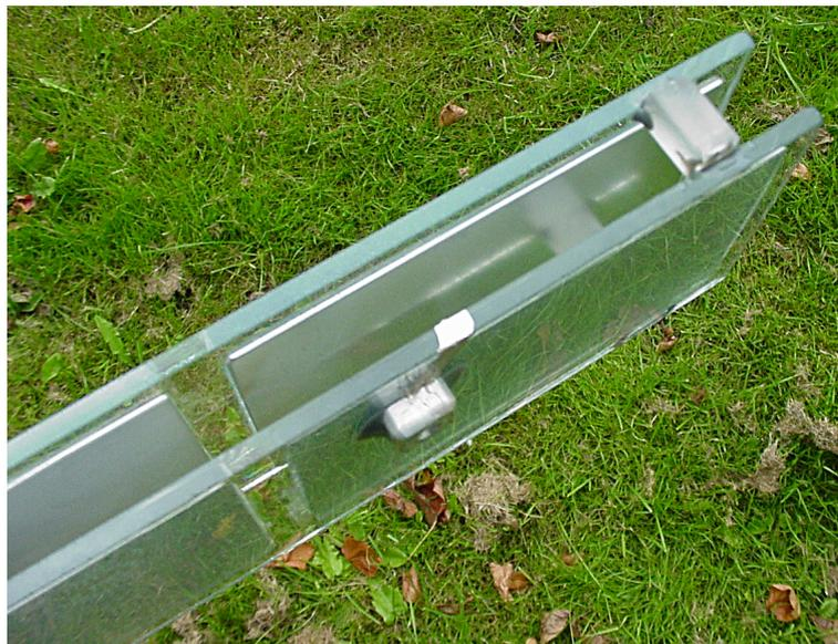
Figure 2.23: A close-up view of the electric field plate assembly.
