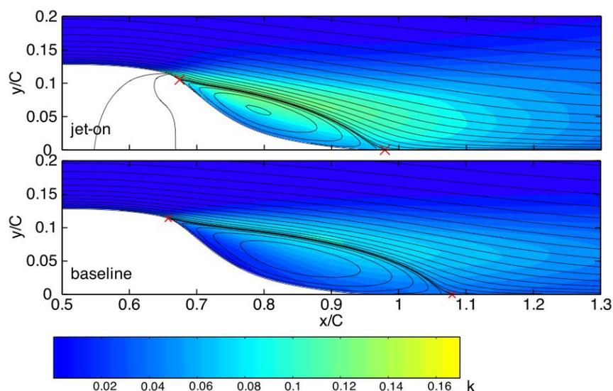
Fig. 3: Time-mean separation zone with (upper) and without (lower) sythetic-jet actuation
