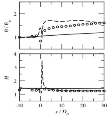
(c) Streamwise evolution of the momentum thickness and the shape factor in the mid-span plane
