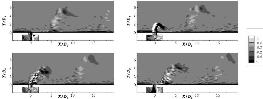
(a) Out-of-plane vorticity in the mid-span plane at various phases
