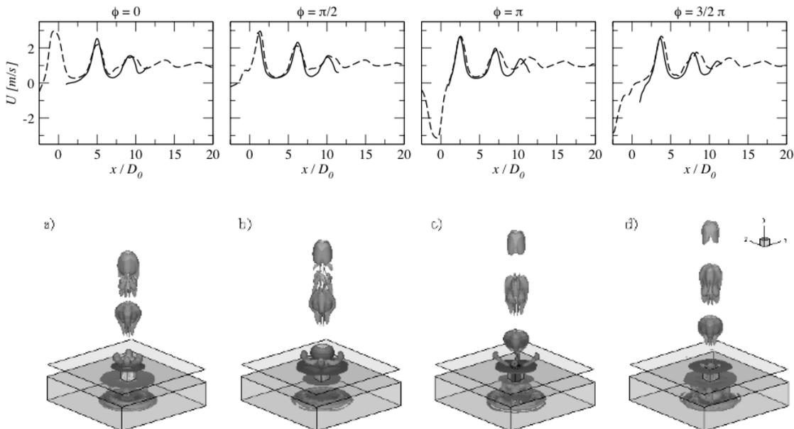
Fig. 5: Isolated synthetic jet ensuing into quiescent surroundings. Above: phase-averaged centre-line velocity, - : PIV data from Garcillan et al. (2004), -- : LES. Below: iso-surfaces of constant vorticity magnitude at the respective phases.
