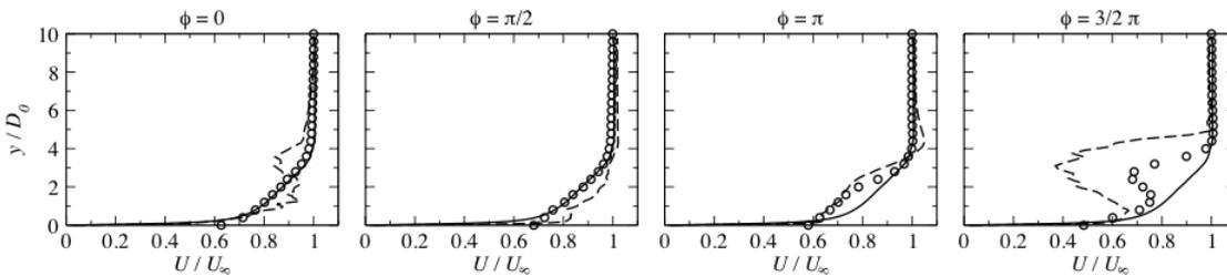
(d) Streamwise velocity profiles at  $x/d_0 = 5$  at various phases.
