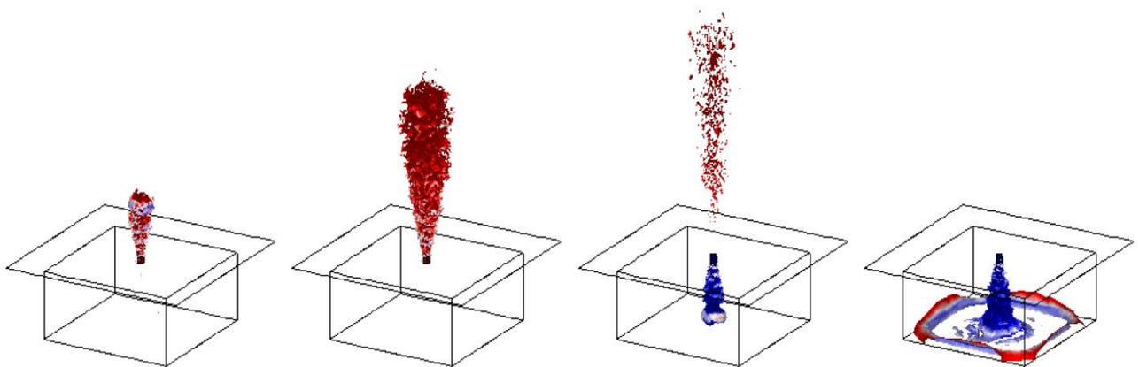
Fig. 1: Synthetic jets in stagnant surroundings – snapshots from large eddy simulations.
